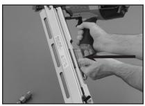
Figure 4. Loading nails into magazine.
